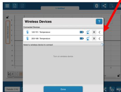
8. Select measurement for left hand axis and choose a temperature sensors, *note the number*
