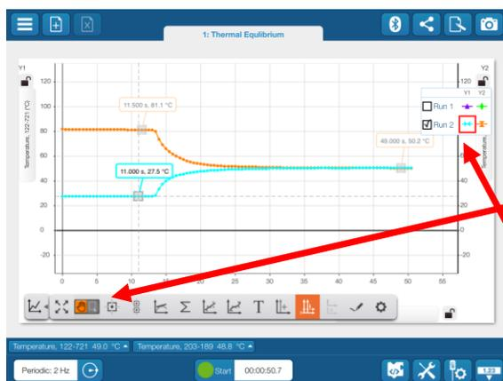
14. When stabilised press the green start button – bottom of screen – and perform your experiment
