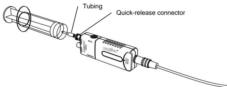
Have students set the volume of a syringe to about 20 mL and then connect it to a data collection system. While monitoring pressure in the digits display, have students observe what happens as they heat the air inside the syringe by holding the syringe in the palm of their hand. Next, have students change the volume of the air in the syringe by pushing the plunger in, compressing the gas. Help students analyze their results by explaining what is happening at the molecular level.
