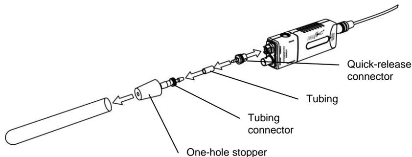
4.  Insert the quick-release connector into the port of the absolute pressure sensor and then turn the connector clockwise until fitting "clicks" onto the sensor (about one-eighth turn).
