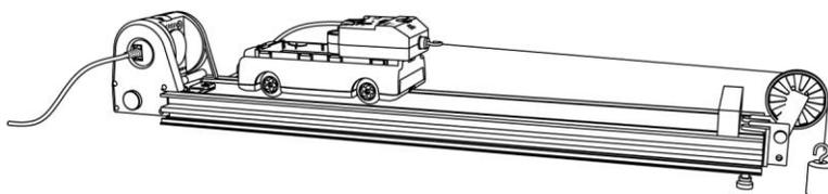
6.  Connect the force sensor to the top of the cart and attach the motion sensor to the end of the dynamics track.
