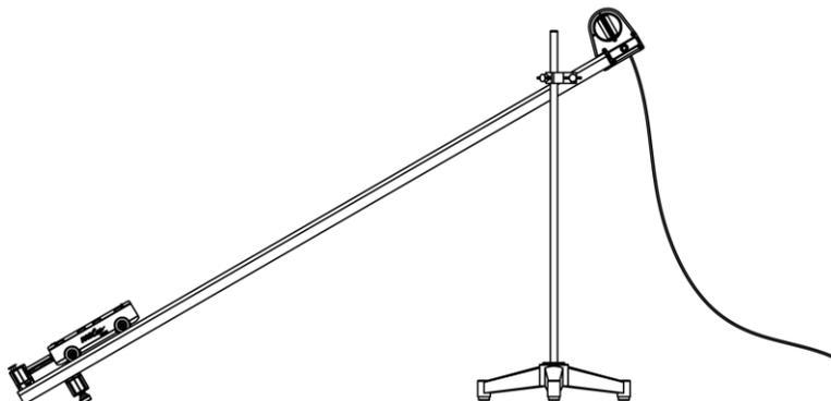
6.  Attach the end stop to the lower end of the dynamics track.
