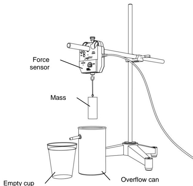
9.  Place a dry cup (catch basin) under the spout of the overflow can.
